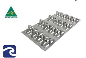
VUETRADE Stainless Steel Tap In Plates are timesaving nail plates with built-in steel 'teeth', ideal for joining timber wall frames and top plates in coastal areas.
